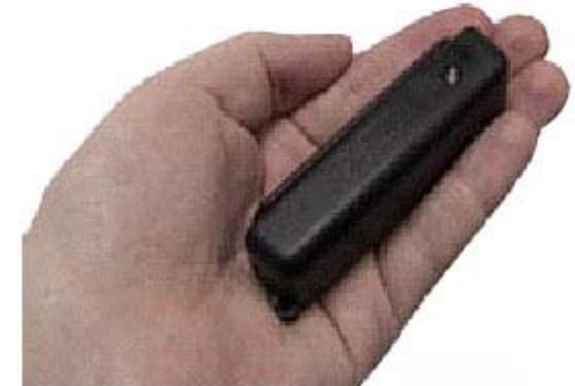
Figure 4: Keycatcher - this is a device that can be connected to a keyboard to record all the keystrokes.
