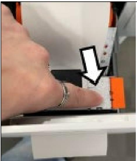
4. Feed the paper through the slot in the printer door.
