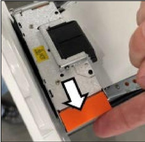
1. Use the opening behind the QR/Barcode scanner to open the printer drawer.
