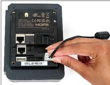
4. Plug the power cable connector into the MDB slave port on the back of the IM30.
