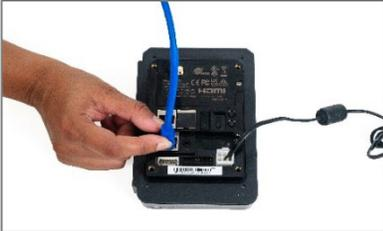
1. Connect your Ethernet cable to the LAN port on the back of the IM30.
