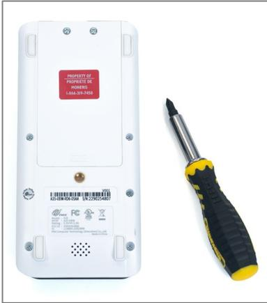
1. Use a screwdriver to remove the two screws located at the top of the plate.
