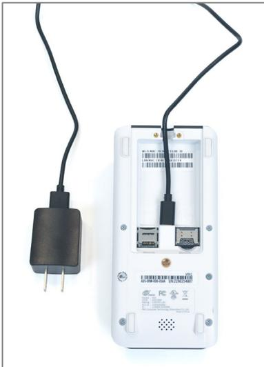
2. Insert the USB C cable into the USB C outlet on the terminal. Make sure the wire is placed securely in the guides located near the exit, at the top of the terminal.
