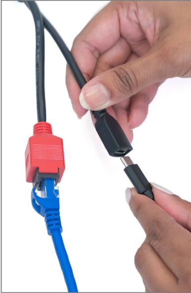
4. Connect the USB C and DC power adapter to the USB C female port on the network and power cable.
