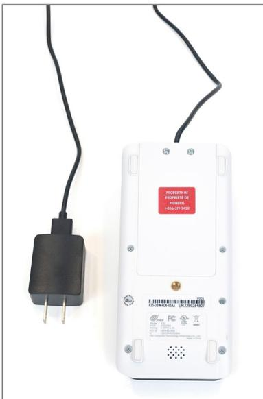
3. Replace the battery plate and screws securely using a screwdriver. Ensure the other end of the cable is securely plugged into the DC adapter.
