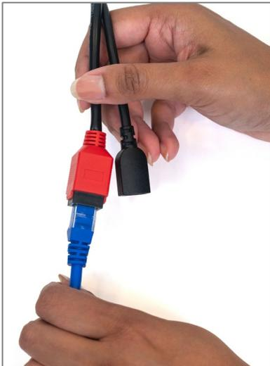
2. Connect your Ethernet cable to the Ethernet outlet attached to the power and network cable.
